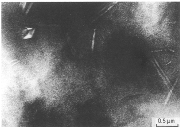
Figure 5 Transmission electron micrograph showing AFt relicts in a large inner product region in a mature OPC paste.
