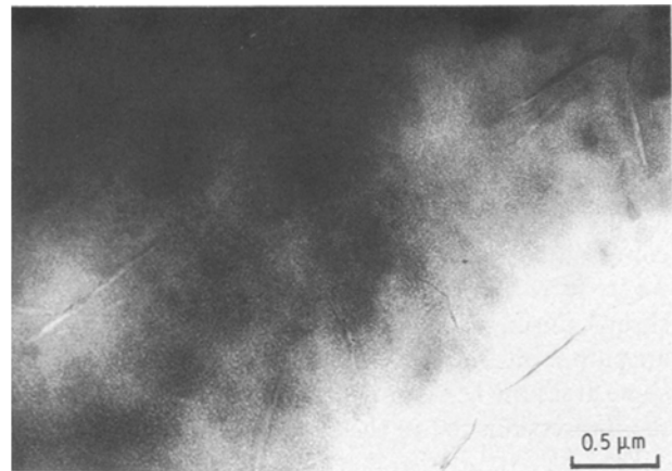
Figure 6 Transmission electron micrograph showing Mg, Al-rich laths in a large inner product region in a mature OPC paste.
