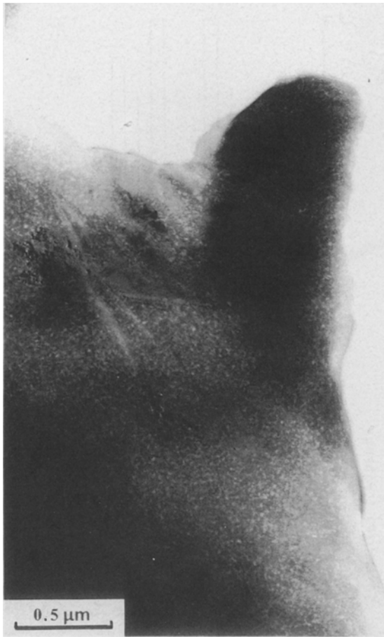
Figure 8 Transmission electron micrograph showing small \text{Ca}(\text{OH})_2 crystals embedded in inner product C-S-H.
