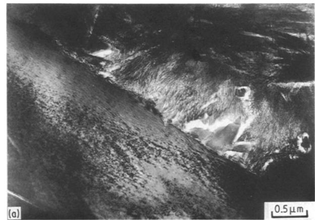
Figure 1 Transmission electron micrographs of an inner product region in a mature hardened Portland cement paste taken (a) soon after bringing the area into the field of view, and (b) \approx 15 s after the first exposure.
